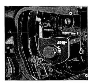
To avoid damage, move the mirror shutter out of the lens port area by turning the knurled wheel (c). If the camera is connected to a power supply, the mirror shutter can also be turned out of the lens port area by pressing the "inching speed" button (26 on back flap).
