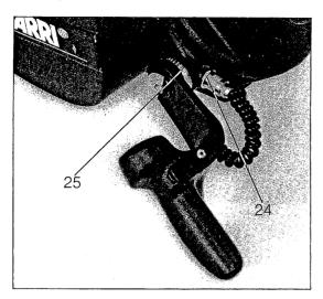
The handgrip with on/off switch is attached to the wedge-shaped rosette (25) of the camera and can be locked in various positions comfortable for the operator. The electrical connection between camera and handgrip is made by the coiled cord which is plugged into the 4-pole flange socket (24).
