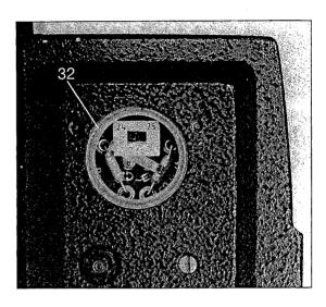
Replace the plastic cover. Obtain a new spare fuse immediately.
