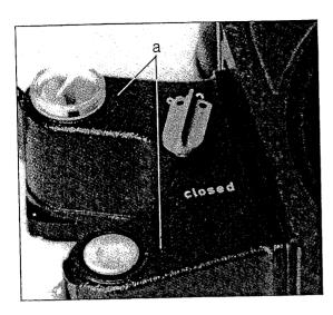
The magazine throat can be cleaned with a soft brush when the captive screws (a) are loosened and the cover (b) is removed. Treat the sprockets with care. Under no circumstances should they be disassembled.
