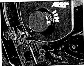
Camera running is indicated by the running control lamp (31 on back flap) on the control panel. The correct functioning of the buckle switch can be verified by operating it while the camera is running.
