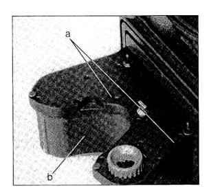
The following parts should also be greased: Magazine lock, the pins of the magazine cover lock (3 each) and the corresponding parts of the magazine cover, camera door lock and tripod thread. Oil the camera door hinges when neccessary.
