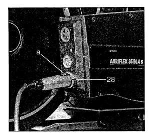
Connect the camera to the battery or the AC sync transformer NSYTR 2, using the cable KCU or the coiled cord KCU Sp. When inserting the 4-pin connecting plug into the flange socket (28), the locking lever (a) must point upwards so that the guide rib of the plug slides exactly into the groove of the flange socket. Ensure correct mechanical locking.
