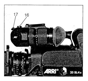
Loosen the clamping screw (17). Press the release button (16) and simultaneously turn the viewfinder approximately 30° clockwise. Now release the button and continue rotating the viewfinder around to its initial viewing position. Through the normal eyepiece, the viewfinder image should appear upside down and laterally inverted. Re-tighten the clamping screw.
