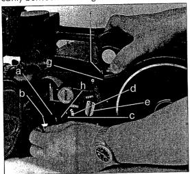
block. Align the film in accordance with the film path marking. Ensure that a perforation of the film loop is engaged by the locating pin at the bottom of the film gate. Turn the magazine lock (e) to "closed". Now push the movement block in the direction of the film gate until there is an audible click. Move the lever of the buckle switch counter-clockwise to its stop position. Then check that the film travels through the movement correctly by turning the knurled knob (h).
