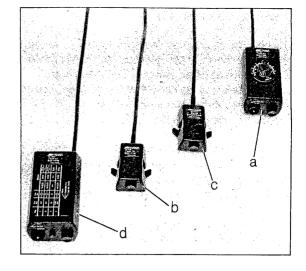
e) The NSYTR 2 AC-synchronizing transformer is used in conjunction with the EXS II for synchronizing the camera with the AC power.
