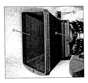
The lightweight matte box is composed of the filter holder (a), the two filter frames (b) and the rectangular sunshade (c). The filter holder is clamped over the front ring of the lens. Lenses with a smaller front diameter require an adapter ring to establish a tight fit. For further information see our Technical Information booklet "Lens Accessory System for ARRIFLEX 35 BL 4/35 BL III/35 III."
