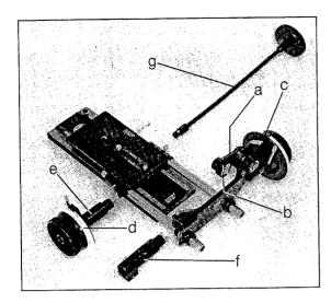
Set the swing arm (a) in either its highest or lowest position. (It swings either up or down to engage the lens focus drive ring, depending on preference). Push the follow-focus unit onto the support rods so that the swing arm is in line with the focus drive ring. Attach the focus gear (b) to the pivoting arm. Swing the arm inward so that the focus gear and lens focusing ring mesh tightly. Fix the pivoting arm into position and then tighten the follow focus to the support rods.
