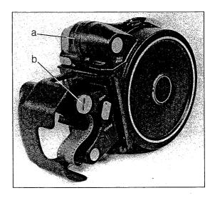
The magazine should be adjusted for the exact film perforation pitch of each different film stock or emulsion batch, before filming.
