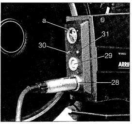
28) The 4-pin flange socket for battery cable (CU or KCU-Sp which supplies power to the :amera.
