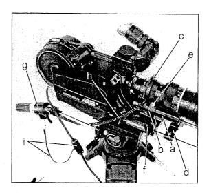
First push the drive-motor inside the mount, ensuring that both motor head and pinion face the camera. Then slide the unit onto the right lens support rod. Slide the lens support guide over the support rods and mount the lens (as described in the previous section "Lens Support").
