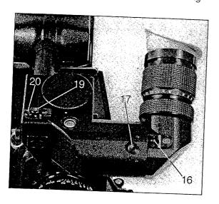
screw (17) and turn the viewfinder to the desired position. Then re-tighten the clamping screw.
