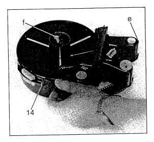
Insert the film into the expandable film core and clamp it in place with the lever (f). Wind the core approximately one turn clockwise. To prevent the film roll from dishing, run a finger around the outer edge of the film core to ensure that the film sits flush with the take-up core. The magazine cover can now be closed.
