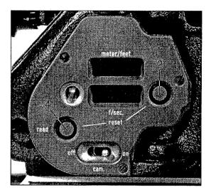
If the "reset" button is not pressed, the amount of film exposed is automatically retained even when the camera is disconnected from the power supply. A 10-year independent lithium battery provides the power for the display unit memory.
