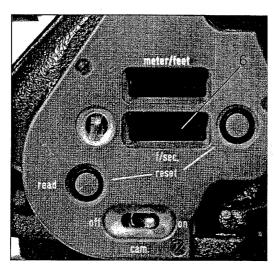
After removal of the plastic cover, the frame rat selector switch (32 on back flap) can be set to the quartz-controlled frame rates of 24 or 25 f (USA: 30 fps). To read or to verify any of the continuously adjustable frame rates from 6 to 50 fps (via VSU), the camera is equipped with digital LED frame rate display (6). Operation is identical with the counter for exposed film located above.
