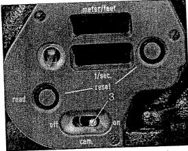
To check the electrical functions, connect the camera to the power supply; then operate the ON/OFF switch [3]. The camera will start to run when the buckle switch (a) is pushed in a counter clockwise direction. While the camera runs up to the selected speed, the red sync control lamp remains visible in the viewfinder. Simultaneously, the out-of-sync warning tone will be heard. Its volume can be adjusted by turning the screw [30 on page 54].
