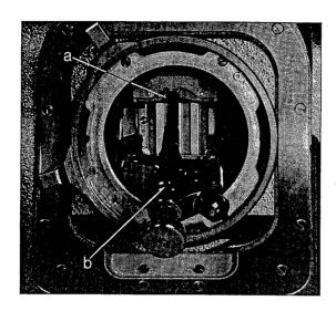
Before changing the focusing screen (a), remove the lens (or cavity cap). Rotate the mirror shutter out of the lens port area, by turning the knurled wheel on the movement block. Using a special forceps (b) or equivalent tool, first pull the focusing screen straight downwards and then out of its holder at a downward angle. Before fitting a new focusing screen, make sure that the focusing screen frame and the holder are completely clean, otherwise the lens may not focus correctly.
