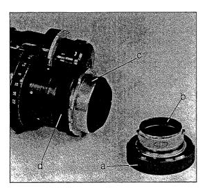
Important: It is not possible to change lenses while the adapter remains in the camera's lens port. Lens and adapter must be removed together from the camera, before the adapter can be fitted to another lens.
