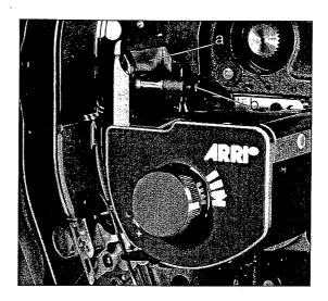
To remove, push the movement block back to the first stop position, pull out the pressure pin (b) and swing the spacer gate out upwards. Remove the spacer gate and clean – do not use objects made of metal or other hard materials. To replace, reverse the procedure.
