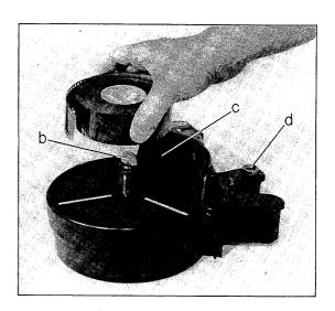
up, and remove the magazine lid. Flip up the hinged clip of the magazine core (b) and insert the sample film roll. Ensure that the guide of the magazine core engages the groove of the plastic film core. Thread the film into the slit (c) as per the film path marking, then return the hinged clip to its horizontal position. The diameter of the magazine core expands when closed, ensuring that the film roll sits snugly and quietly on the feed-side spindle.
