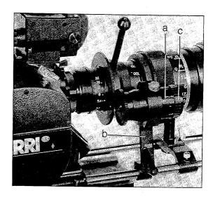
The fluid drive (a) enables smooth manual zooming. Like the servo zoom drive, it is secured in the motor mount (b), swung into the toothed drive ring on the lens and secured in position. The friction effect can be graduated as desired via the setting ring (c).
