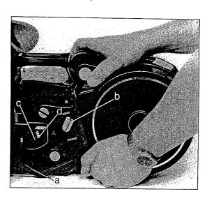
To remove a magazine with fully exposed roll, first open the camera door and, after releasing the lock (a), push back the movement block in the direction of the magazine into the lock position. Turn the magazine lock (b) to "open" and pull the magazine out of the dovetail guide of the camera.
