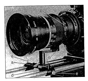
To assemble the two-part lens support, first slide the lens support guide (a) onto the bridge plate support rods. Mount the lens with its lens support ring (b), on the camera. While supporting the lens, slide the lens support guide directly underneath the spacer rod of the lens support ring (b). Tighten the knurled screw (d) to secure the lens support, then tighten the knurled screws (e) that fix the support to the lens rods. Finally tighten the clamping lever (f) in position.
