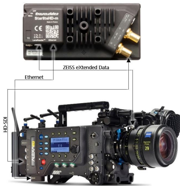
Connection plan with Alexa SXT, LF and 65
