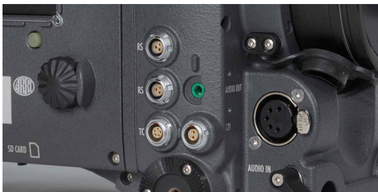
Fig. 4: 24 V outputs (RS) and 12 V output
