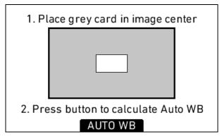
The AUTO WB value is always stored as the first entry of the WB list. This entry is overwritten every time an automatic white balance is performed. To save an AUTO WB value, press ADD after the successfull calulation, and press the wheel twice. The AUTO WB result will be saved as a user value in the WB list.
