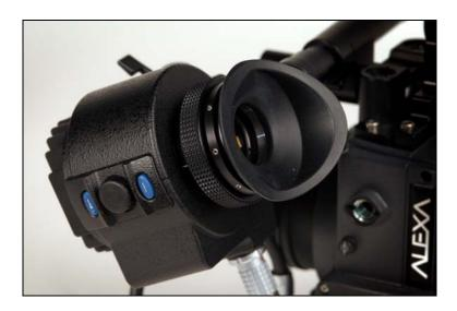
The EVF-1 employs an LCOS imaging device together with a temperature stabilized LED light source to provide an accurate and bright view of the sensor image under all operating conditions. The viewfinder is calibrated to match the image of the camera's HD outputs.
