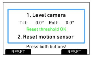
Figure 85: Motion sensor reset screen
