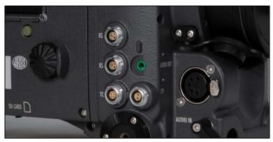
Figure 10: 24 V outputs (RS) and 12 V output
