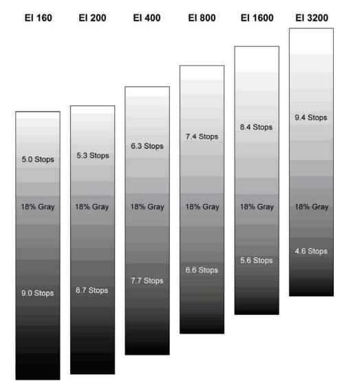
Figure 42: Graphical comparison of latitude at different exposure indexes
