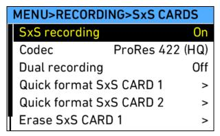
SxS recording Switches SxS recording on or off. With SxS
