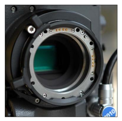
Figure 82: Lens adapter PL-Mount LA-PL-2 (with LDS)
