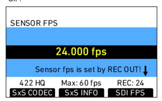
Figure 34: Fps screen with linked sensor fps
