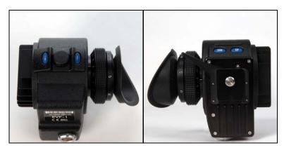
The EVF buttons are locked whith the camera UI by pressing the LOCK button on the camera left or right side until the lock timer has elapsed. On the right side the timer is shown as a countdown on the display. The locked controls are visualized by a lock icon. On the left side the locked controls are visualized by a blue LED next to the LOCK button.
