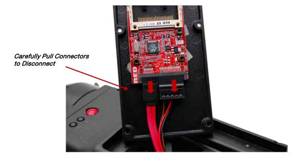
5. Remove the CF Module from the camera body.
